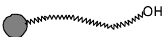
Figure 3.2 General structure of a monol (oligo polyol with only one hydroxyl group/mol)
