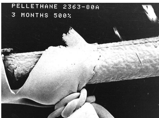
FIGURE 24.10 Pellethane failure after three months implantation.
