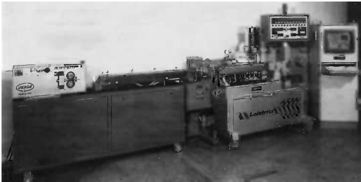
FIGURE 17.3 Micro-18-mm modular/multimode twin-screw extruder with screw pump, downstream tube system, and ECS controls. (From American Leistriz Extruder Corp.)
