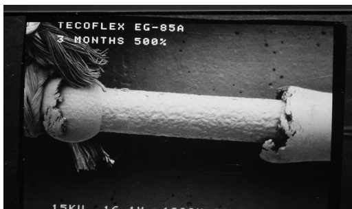
FIGURE 24.9 Tecoflex failure after three months implantation.
